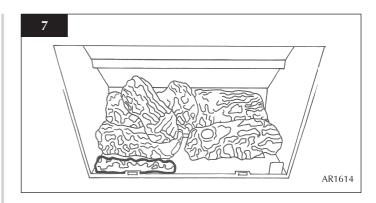
7.6 Place the second ash panel to the right of the first, with the pointed end of the panel fitting into the V shape. This panel should locate on the screw holes of the burner skin. Ensure that both logs are horizontal to the burner ports.
